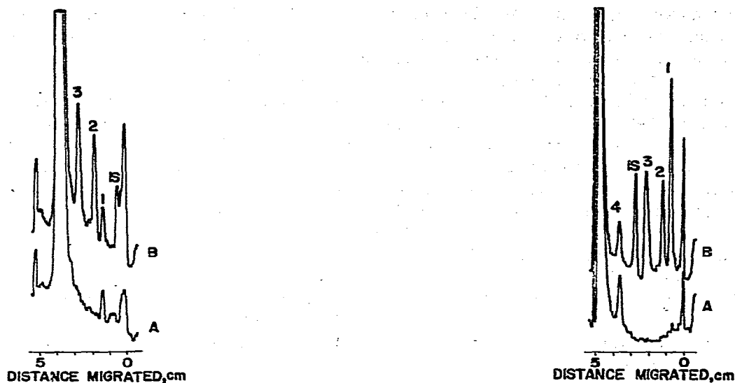
Fig. 1. Chromatogram of drugs separated using solvent system I. IS = internal standard; 1 = caffeine; 2 = lidocaine; 3 = diphenylhydantoin. A, serum blank; B, serum to which drugs have been added.
